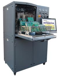
Our de-fluxing systems are available in a variety of discharge and throughput configurations and provide wash, rinse, cleanliness monitoring, drying and SPC processes. Trident is capable of removing residues, including all lead and lead-free residues from low stand-off component spaces. These systems can be configured to match specific production needs.
